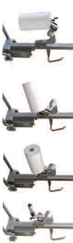
Reel Handling Vertical to Horizontal Via the Core
