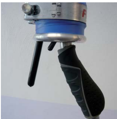
VQL with ergonomic one-hand-control
