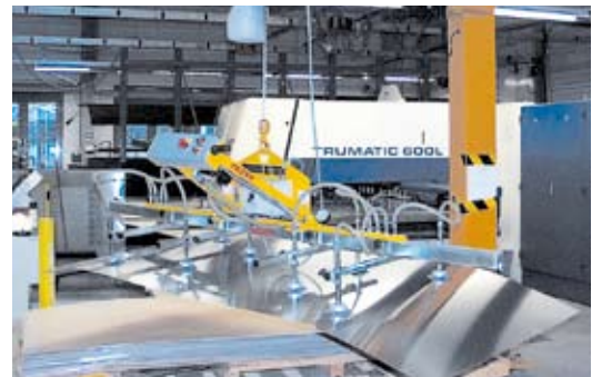
Handling of large sheet metal boards
