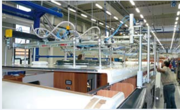
VacuBoy during the assembly of car roofs
