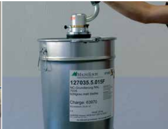
Single suction foot in bellows design
