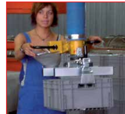
Mechanical gripper for crates with suspension clips
