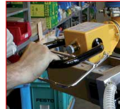
Control housing with tilting lever for intuitive and simple operation
