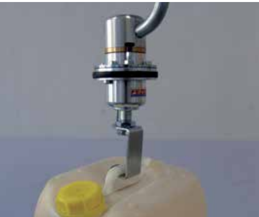
Canister gripper with balancer valve
