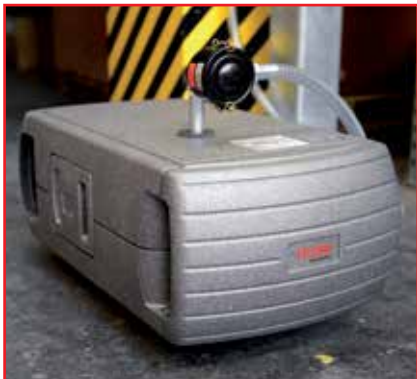
Vacuum generator with silencer box to reduce the noise level
