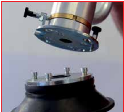
Quick-change coupling with bayonet connector and arrests
