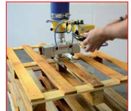
Pallet gripper with pneumatically adjustable undergrippers
