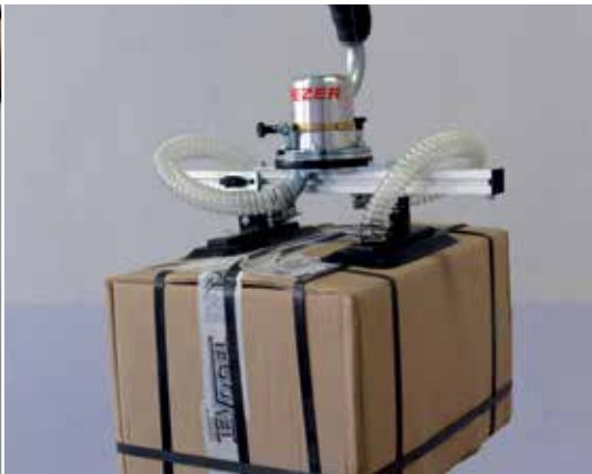
Double suction foot with adjustable suction pads on main beam
