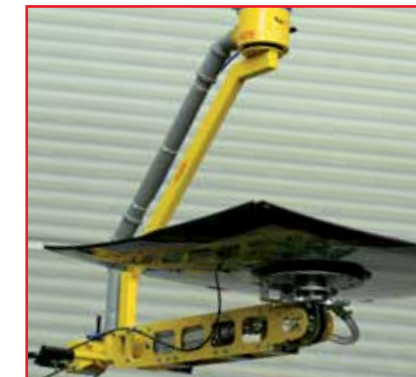
Pneumatical turn-over feature for flipping workpieces over by 180°
