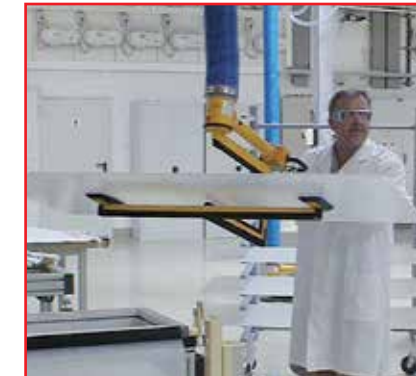
Mechanical gripper as undergripper for glass panes
