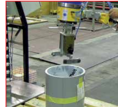
Pneumatic gripper for handling coils or tubes
