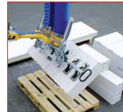
Special suction foot for simultaneous handling of several concrete stones
